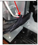
excess wires are bundled away from the axial fan blade
